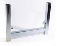
Manufactured from 50 x 50 x 2.5mm SHS section with 50 x 50mm flat plate bent to lock the tube in place Size 1 - Storage capacity of 48no tubes and stackable 5no units high Size 2 - Storage capacity of 72no tubes and stackable 3no units high Supplied galvanised finish
