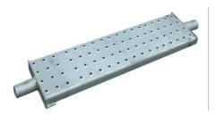
Fabricated stair tread complete with 48.3mm nominal tubular spigot welded to RSA cap at each end, surface finish with a series of pierced holes for grip.
